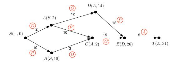
The ship can be assembled in 31 units of time along SADET, that is, by first detaching and sorting the pieces, then gluing, painting and applying the decals.
